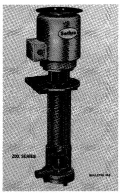
The ZDX series of vertical CPVC pumps are now available in five sizes with flow capacities to 80 gpm at 200 F. Each model is designed with wide upper and lower liquid level limits and constructed without bearings, seals, or wearing parts. More information: Sethco Mfg. Corp., One Bennington Ave., Freeport, NY 11520.
